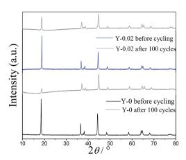
Fig. 11 PXRD patterns of the Y-0 and Y-0.02 materials before cycling and after 100 cycles.
