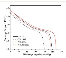
Fig. 8 Discharge curves of the Y-O and Y-O.02 samples after the 1st and 100th cycle at a rate of 1C.
