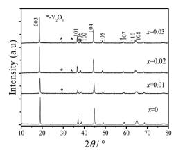
Fig. 1 XRD patterns of the LiNi<sub>0.5</sub>Co<sub>0.2-x</sub>Mn<sub>0.3</sub>Y<sub>x</sub>O<sub>2</sub> materials.
