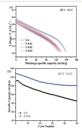
Fig. 10 (a) Discharge curves of the samples at a rate of 0.2C at -20 °C and (b) the cycling performance curves of the samples Y-0 and Y-0.02 at a rate of 0.2C at -20 °C.
