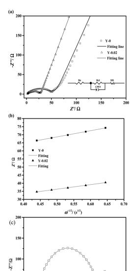
Fig. 14 Electrochemical impedance measurements of the Y-O and Y-0.02 samples: (a) Nyquist curves and fitting-figures of both samples, (b) graphs of Z' against  $\omega^{-1/2}$  for both samples. (c) Nyquist plots of the Y-0 and Y-0.02 samples after 50 cycles.
