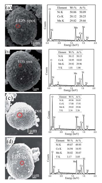
Fig. 4 SEM images of the materials (a) Y-0, (b) Y-0.01, (c) Y-0.02, and (d) Y-0.03 and the corresponding EDS images.
