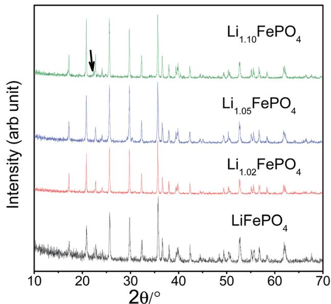
Fig. 1 Representative XRD patterns recorded with all the four LFP-based samples (*i.e.*, A, B, C and D; or starting Li-contents corresponding to  $x = 1.0, 1.02, 1.05$  and  $1.10$  in  $\text{Li}_x\text{FePO}_4$ ).
