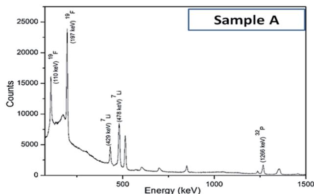
Fig. 3 Typical gamma-ray spectrum of sample A, as obtained with proton induced gamma emission (PIGE) technique.
