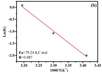
Fig. 11 The effect of reaction temperature on RhB degradation over the CoFe<sub>2</sub>O<sub>4</sub>/GO catalyst (a); the Arrhenius plot with linear regression (b); reaction conditions: [RhB] = 0.03 mmol L<sup>-1</sup>, amount of catalyst = 10 mg and 0.1 g L<sup>-1</sup> of oxone at different temperatures.
