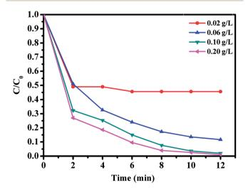
Fig. 10 Effect of oxone concentration on RhB degradation over CoFe<sub>2</sub>O<sub>4</sub>/GO. Reaction conditions: [RhB] = 0.03 mmol L<sup>-1</sup>, amount of catalyst = 10 mg, T = 25 °C.
