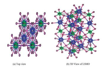
Fig. 5 (a) Top view and (b) 3-dimensional structure of the prepared LSMO sample.
