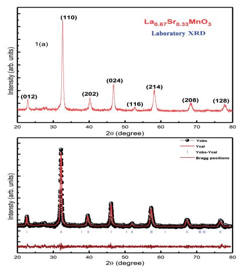
(a) RT-XRD spectrum of La<sub>0.67</sub>Sr<sub>0.33</sub>MnO<sub>3</sub> (LSMO) and (b) Rietveld refinement of the XRD data of LSMO
