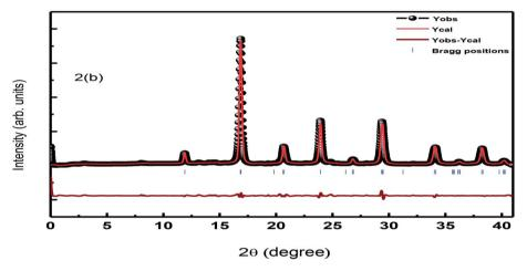
Fig. 2 (a) SR-XRD of LSMO and (b) Rietveld refinement of the SR-XRD pattern of LSMO.
