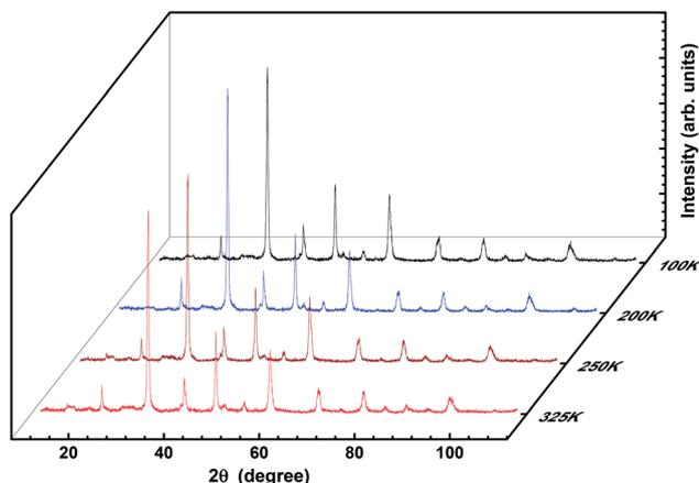
Fig. 3 3D plot of temperature-dependent XRD of LSMO.
