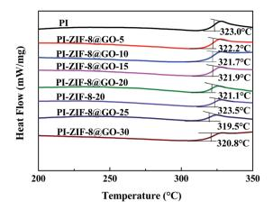
Fig. 9 DSC curves obtained for the membranes
