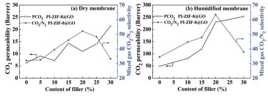
Fig. 12 Comparison of the mixed gas separation performance observed for the dry and humidified membranes: (a) CO<sub>2</sub> permeability and CO<sub>2</sub>/  $N_2$  selectivity observed for the dry membranes; (b)  $CO_2$  permeability and  $CO_2/N_2$  selectivity observed for the dry membranes with the ZIF-8@GO based MMMs (1.0 bar, 30 °C).
