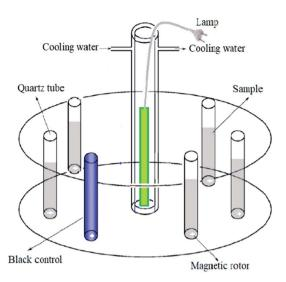
Fig. 1 A schematic of the experimental setup
