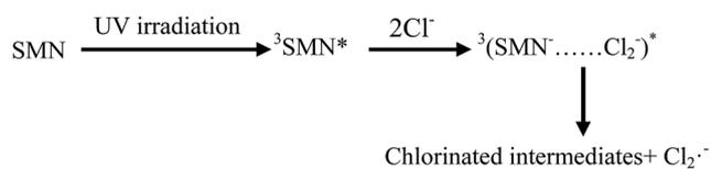
Scheme 2 Reaction pathway of SMN induced by chloride ion.
