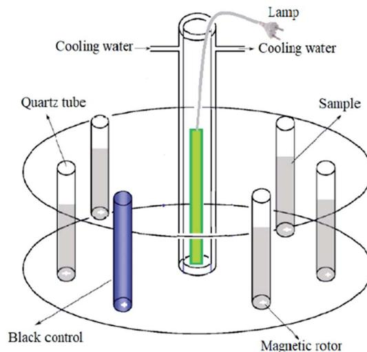
Fig. 1 A schematic of the experimental setup.
