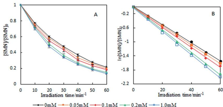
Fig. 6 Effects of  $\text{NO}_3^-$  on degradation ratio (A) and kinetics (B) of SMN photolysis.
