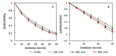
Fig. 5 Effects of Cl<sup>-</sup> on degradation ratio (A) and kinetics (B) of SMN photolysis
