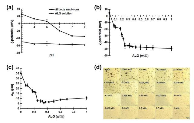
Fig. 2 The ζ-potential of pure OB emulsions and pure ALG solution (a); ζ-potential (b), mean particle diameter ( $d_{43}$ ) (c) and the microscopic structure (d) of OB emulsions each with 1.0 wt% oil bodies and different concentrations of ALG. The continuous phase of the emulsions is 50 mM sodium phosphate and pH is 4.5.
