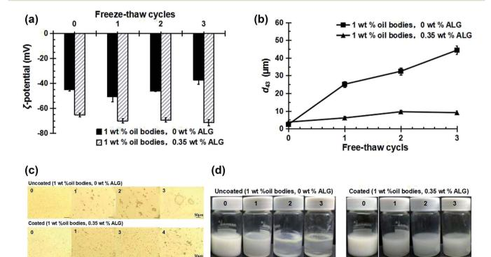
Fig. 7 Effect of freezing—thawing cycling on  $\zeta$ -potential (a); mean particle diameter ( $d_{43}$ ) (b); the microscopic structure (c) and the creaming stability (d) of uncoated (1 wt% oil bodies, 0 wt% ALG) and coated (1 wt% oil bodies, 0.35 wt% ALG) OB emulsions at pH 7. The oil bodies were dispersed in 50 mM sodium phosphate buffer solution. The creaming observation was made after storage at 22  $\pm$  2 °C for 7 days."0, 1, 2, 3" represents the number of the freezing—thawing cycles.
