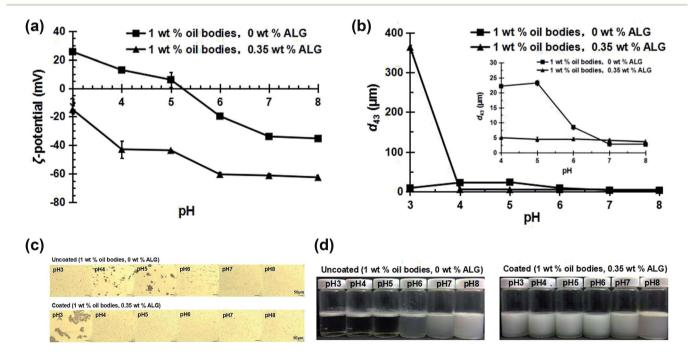
Fig. 5 pH effect on  $\zeta$ -potential (a); mean particle diameter ( $d_{43}$ ) (b); the microscopic structure (c) and the creaming stability (d) of uncoated (1 wt% oil bodies, 0 wt% ALG) and coated (1 wt% oil bodies, 0.35 wt% ALG) OB emulsions. The oil bodies were dispersed in 50 mM sodium phosphate buffer solution. The creaming observation was made after storage at 22  $\pm$  2 °C for 7 days.
