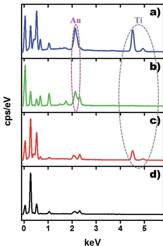
Fig. 2 EDX spectrum of the TiO<sub>2</sub> NW/PAPBA–Au TNC, PAPBA–Au NC, TiO<sub>2</sub> NW/PAPBA NC, pristine PAPBA.
