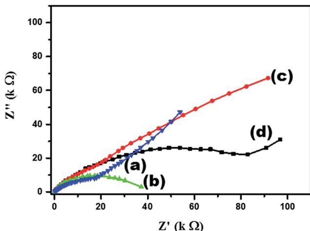
Fig. 6 Nyquist plots ( $Z''$  versus  $Z'$ ) of GCE/TiO<sub>2</sub> NW/PAPBA–Au TNC (a), GCE/PAPBA–Au NC (b), GCE/TiO<sub>2</sub> NW/PAPBA NC (c) and GCE/pristine PAPBA (d) electrodes recorded in 5 mM of Fe(CN)<sub>6</sub><sup>3-/4-</sup> (0.1 M KCl).
