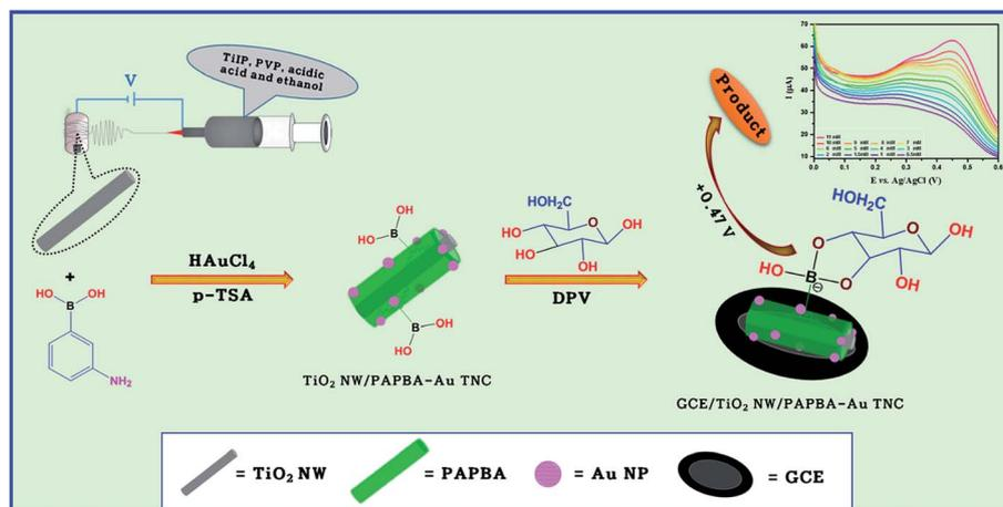
Scheme 1 Schematic diagram of the preparation of TiO<sub>2</sub> NW/PAPBA–Au TNC and electrochemical performance towards glucose detection.
