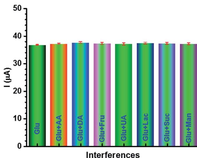
Fig. 9 DPV current responses at the GCE/TiO<sub>2</sub> NW/PAPBA-Au TNC electrode for 0.1 M PBS (pH 7.0) containing 1.0 mM glucose in the presence of 1.0 mM each ascorbic acid (AA), uric acid (UA), dopamine (DA), fructose (Fru), lactose (Lac), sucrose (Suc) and mannose (Mon). Scan rate: 50 mV s<sup>-1</sup>, pulse amplitude: 50 mV, pulse width: 50 ms.
