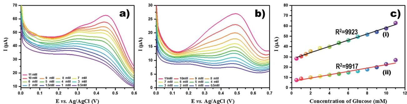
Fig. 8 DPV for various glucose concentration (0.5 to 11 mM) at (a) GCE/TiO<sub>2</sub> NW/PAPBA-Au TNC and (b) GCE/PAPBA-Au NC modified electrodes in phosphate buffer (pH 7). Scan rate: 50 mV s<sup>-1</sup>, pulse amplitude: 50 mV, pulse width: 50 ms. (c) The plot of peak current *I* (mA) versus concentration glucose at (i) GCE/TiO<sub>2</sub> NW/PAPBA-Au TNC and (ii) GCE/PAPBA-Au NC modified electrodes.
