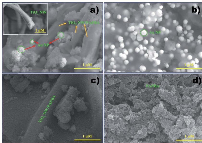
Fig. 1 FE-SEM images of (a) TiO<sub>2</sub> NW/PAPBA–Au TNC, (inset: image of TiO<sub>2</sub> NW) (b) PAPBA–Au NC, (c) TiO<sub>2</sub> NW/PAPBA NC, (d) pristine PAPBA.
