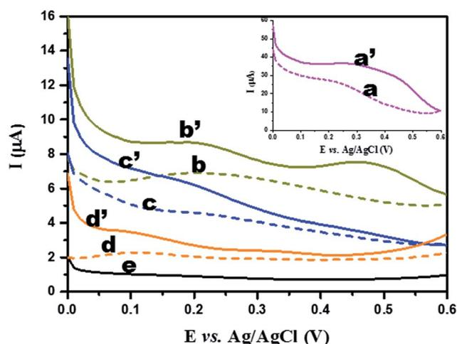
Fig. 7 DPV of glucose oxidation of GCE/TiO<sub>2</sub> NW/PAPBA–Au TNC (a and a'), GCE/PAPBA–Au NC (b and b'), GCE/TiO<sub>2</sub> NW/PAPBA NC (c and c'), GCE/pristine PAPBA (d and d') and bare GCE (e) in 1 mM glucose + 0.1 M PBS solution (solid lines; a'–d') and absence of glucose (dashed lines; a–e). Scan rate: 0.05 V s<sup>-1</sup>, pulse amplitude: 0.05 V, pulse width: 50 ms.
