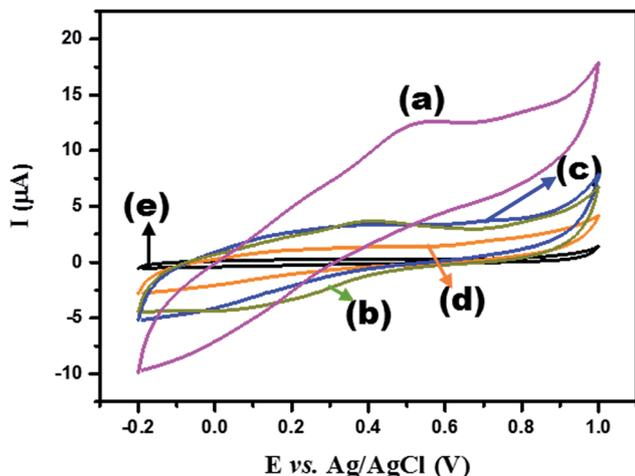
Fig. 5 CV curves of GCE/TiO<sub>2</sub> NW/PAPBA–Au TNC (a), GCE/PAPBA–Au NC (b), GCE/TiO<sub>2</sub> NW/PAPBA NC (c), GCE/pristine PAPBA (d) and bare GCE (e) electrodes recorded in 0.1 M PBS (pH 7) solution. Scan rate: 50 mV s<sup>-1</sup>.
