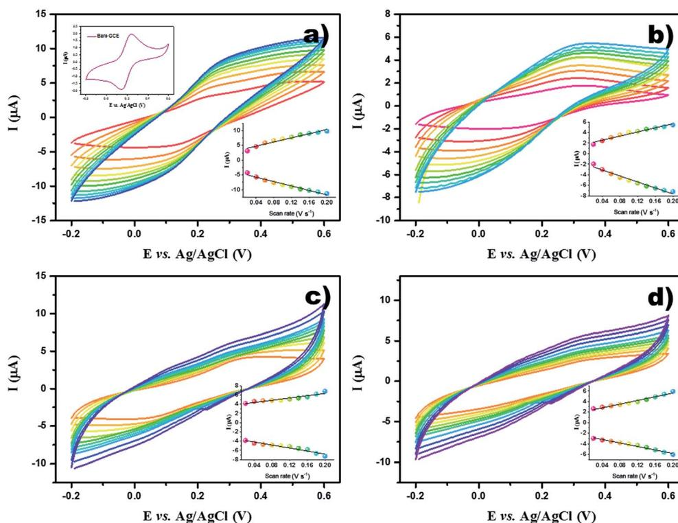
Fig. 4 CV curves for  $5$  mM of Fe(CN)<sub>6</sub><sup>3-/4-</sup> ( $0.1$  M KCl) at different scan rate from  $0.02$  V s<sup>-1</sup> to  $0.20$  V s<sup>-1</sup> at the modified electrodes GCE/TiO<sub>2</sub> NW/PAPBA–Au TNC (a), GCE/PAPBA–Au NC (b), GCE/TiO<sub>2</sub> NW/PAPBA NC (c), GCE/pristine PAPBA (d) and bare GCE (a, inset).
