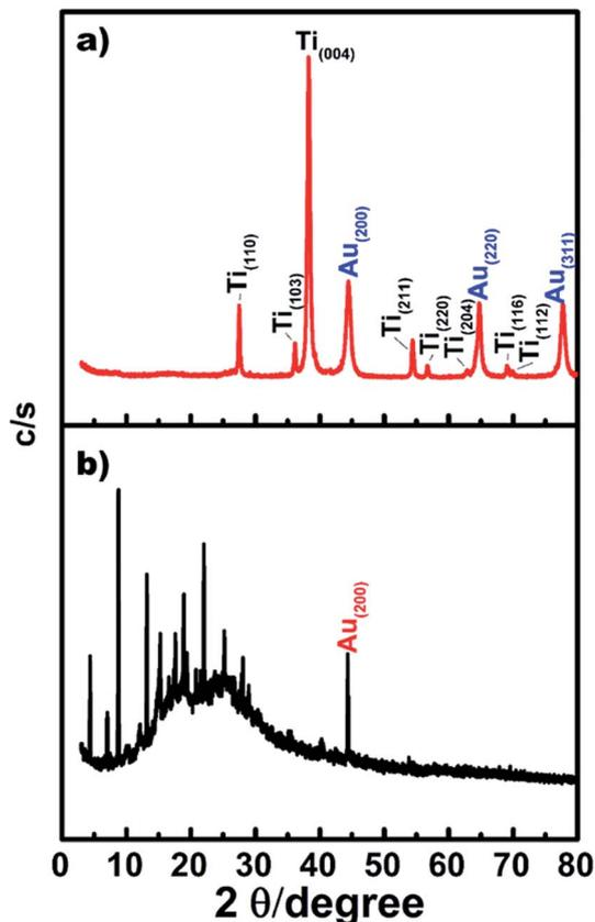
Fig. 3 XRD pattern of the TiO<sub>2</sub> NW/PAPBA–Au TNC, PAPBA–Au NC.
