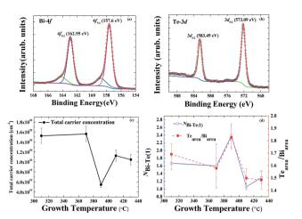
Fig. 3 XPS of (a) Bi-4f core-level spectra and (b) Te-3d core-level spectra of the  $Bi_2Te_3$  thin film grown at 390 °C. (c) Total carrier concentration of the  $Bi_2Te_3$  films as a function of the growth temperature measured by Hall measurement. (d) The Te/Bi ratio of the  $Bi_2Te_3$  thin films as a function of the growth temperature.
