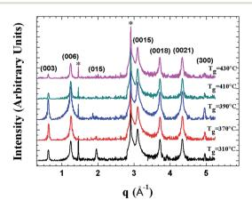
Fig. 1 XRD curves of several Bi<sub>2</sub>Te<sub>3</sub> epilayers grown with MBE at substrate temperature  $T_{\rm q}$  from 310 to 430 °C. In this  $T_{\rm q}$  range, XRD curves of Bi<sub>2</sub>Te<sub>3</sub> samples clearly show features related to a singlecrystal Bi<sub>2</sub>Te<sub>3</sub> epilayer that is (0001)-oriented on the sapphire (0001) substrate (indicated by \*).
