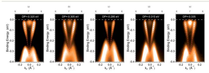
Fig. 2 Band structure of  $Bi_2Te_3$  at various  $T_g$ : (a) 310 °C (DP = -0.32 eV). (b) 370 °C (DP = -0.305 eV). (c) 390 °C (DP = -0.295 eV). (d) 410 °C (DP = -0.315 eV). (e) 430 °C (DP = -0.335 eV). All spectra were recorded along the  $\Gamma$ -K direction. The panels show the ARPES intensity maps. The surface states, valence band and conduction band of the bulk states are denoted SS, VB and CB, respectively.
