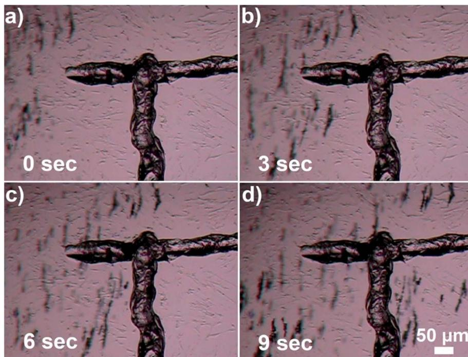
Fig. 5 Magnet-controlled movement of Au nanocages-covered magnetic microbeads towards T-marked area. (a) 1  $\mu\text{l}$  solution of Au nanocages-decorated microbeads is dropped away from the marker. Next, the external magnet is placed approximately 1 cm away from the sample. (b)–(d) Gradual movement of the magnetic beads into the desired area.
