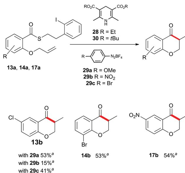
**Scheme 6** Indirect acyl radical generation and cyclization with electron-deficient substrates. <sup>a</sup> Yield based on recovered starting material.
