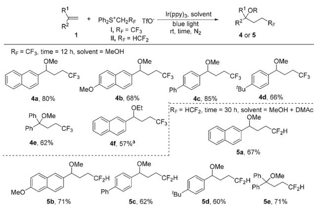
**Scheme 3** Methoxytri- and methoxydi-fluoroethylation of alkenes. Isolated yields. Reaction conditions: Substrate **1a** (0.5 mmol), reagent **I** or **II** (2 equiv.) and  $\text{Ir}(\text{ppy})_3$  (2 mol%) in DMAc (3 mL) or DMAc/MeOH ( $v/v = 2\text{ mL}/1\text{ mL}$ ) irradiated with blue LEDs at room temperature for 12 h or 30 h. <sup>a</sup> EtOH/DMAc ( $v/v = 1\text{ mL}/2\text{ mL}$ ) was used as the solvent instead of MeOH to obtain product **4f**.
