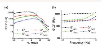
Fig. 6 Rheology experiment of the metallogels of 1: (a) amplitude sweep and (b) frequency sweep.
