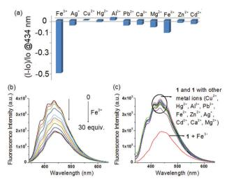
Fig. 7 (a) Change in fluorescence ratio ( $\lambda_{\rm ex}$  = 330 nm) of **1** (c = 2.5  $\times$  10<sup>-5</sup> M) at 434 nm upon addition of 30 equiv. amounts of different metal ions (c = 1.0  $\times$  10<sup>-3</sup> M) in CHCl<sub>3</sub>/CH<sub>3</sub>OH (3:1, v/v); change in fluorescence intensity of **1** upon addition of 30 equiv. amounts of (b) Fe<sup>3+</sup> and (c) different metal ions.
