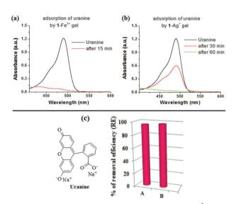
Fig. 10 Change in absorbance of uranine solution ( $c = 3 \times 10^{-5}$  M) before and after adsorption on (a) 1-Fe<sup>3+</sup> gel and (b) 1-Ag<sup>+</sup> gel. (c) The bar plot shows the respective dye adsorption data; adsorption of uranine by (A)  $1-Fe^{3+}$  and (B)  $1-Ag^{+}$  gels.
