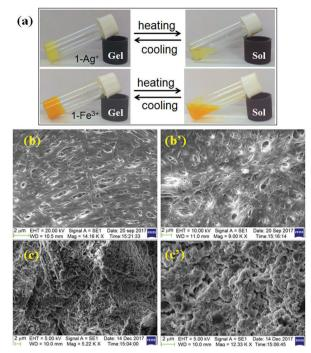
Fig. 4 (a) Photograph showing the thermo reversibility of  $Ag^+$ -induced and  $Fe^{3+}$ -induced gels of **1** (top) and SEM images of the metallogels of **1** with  $Fe^{3+}$  (b and b') and  $Ag^+$  ions (c and c') (below).
