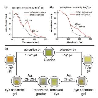
Fig. 11 Comparison of normalized UV-vis spectra of (a) 1-Fe<sup>3+</sup> gel and (b) 1-Ag<sup>+</sup> gel, before and after adsorption of uranine and (c) photograph showing the recyclability of the uranine adsorption process.
