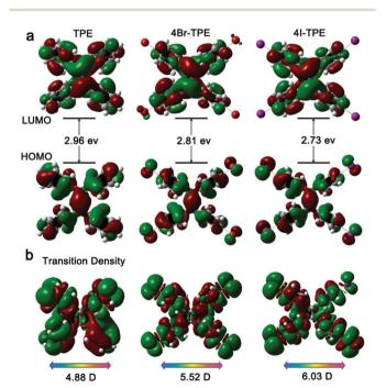
Fig. 4 (a) Calculated electronic structures and bandgaps of TPE, 4Br-TPE and 4I-TPE; (b) the transition densities corresponding to  $S_0-S_1$  of TPE, 4Br-TPE and 4I-TPE.
