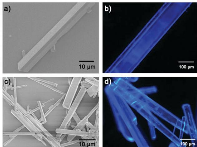
**Fig. 2** Morphologies of 4Br-TPE and 4I-TPE microcrystals. (a) SEM image of microrod 4Br-TPE; (b) fluorescent microscopic image of 4Br-TPE; (c) SEM image of 4I-TPE microrod; (d) fluorescent microscopic image of 4I-TPE.
