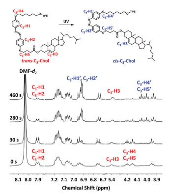
Fig. 6 <sup>1</sup>H NMR (400 MHz) of trans-C<sub>3</sub>-Chol gel in DMF- $d_7$  (c = 0.45 mM) under UV irradiation at 365 nm (0.25 mW cm<sup>-2</sup>) as a function of irradiation time.
