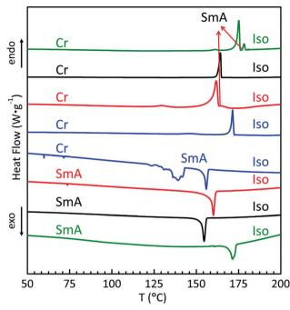
Fig. 1 DSC thermograms of  $trans-C_0$ -Chol (green lines),  $trans-C_1$ -Chol (black lines),  $trans-C_3$ -Chol (red lines) and  $trans-C_5$ -Chol (blue lines) upon the first heating (4 upper curves) and first cooling (4 lower curves) cycle at a rate of 2 °C min<sup>-1</sup>. Samples are solids obtained by recrystallization after synthesis.
