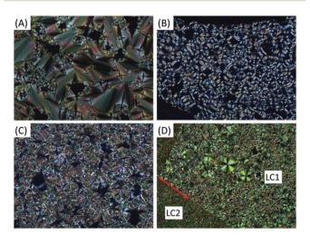
Fig. 2 Textures of trans- $C_n$ -Chol observed by POM upon cooling from isotropic phase. (A) trans- $C_0$ -Chol at 25 °C; (B) trans- $C_1$ -Chol at 25 °C; (C) trans- $C_3$ -Chol at 25 °C; (D) trans- $C_5$ -Chol at 145 °C (the second phase LC2 started to grow from the left side). These typical fan-shaped textures indicate SmA phase. In (D) LC1 is SmA, while LC2 is a crystalline phase (see text).
