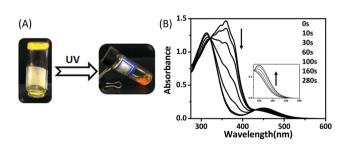
Fig. 5 (A) Photos showing gel-sol transition of trans-C5-Chol in DMF (c = 62 mM) after 15 min of UV irradiation (90 mW cm<sup>-2</sup>, 365 nm). (B) UV-Vis spectra of  $trans-C_5$ -Chol in DMF solution (c = 0.1 mM) with different UV irradiation time (0.25 mW cm<sup>-2</sup>, 365 nm).
