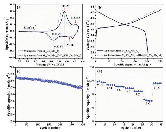
Fig. 5 (a) CV curves (0.1 mV s<sup>-1</sup>) and (b) initial charge-discharge profiles (0.28C) of  $LiNi_{0.8}Co_{0.1}Mn_{0.1}O_2$  prepared from  $Ni_{0.8}Co_{0.1}Mn_{0.1}O_x$  and LiNi<sub>0.8</sub>Co<sub>0.1</sub>Mn<sub>0.1</sub>O<sub>2</sub> spheres in the rate range of 0.1–10C.
