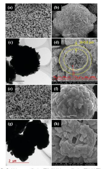
Fig. 3 (a) Low-magnification SEM, (b) high-magnification SEM, (c) TEM and (d) cross-sectional SEM images of the holistic  $Ni_{0.8}Co_{0.1}Mn_{0.1}(OH)_2$ @  $Ni_{0.8}Co_{0.1}Mn_{0.1}O_x$  precursor. (e) Low-magnification SEM, (f) high-magnification SEM, (g) TEM and (h) cross-sectional SEM images of the LiNi<sub>0.8</sub>Co<sub>0.1</sub>Mn<sub>0.1</sub>O<sub>2</sub> microspheres
