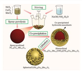
Scheme 1 Schematic diagram of the synthesis process for the LiNi<sub>0.8</sub>-Co<sub>0.1</sub>Mn<sub>0.1</sub>O<sub>2</sub> microspheres.
