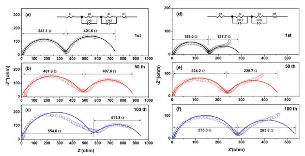
Fig. 6 EIS of LiNi<sub>0.8</sub>Co<sub>0.1</sub>Mn<sub>0.1</sub>O<sub>2</sub> prepared from (a-c) Ni<sub>0.8</sub>Co<sub>0.1</sub>Mn<sub>0.1</sub>O<sub>x</sub> and from (d-f) Ni<sub>0.8</sub>Co<sub>0.1</sub>Mn<sub>0.1</sub>(OH)<sub>2</sub>@Ni<sub>0.8</sub>Co<sub>0.1</sub>Mn<sub>0.1</sub>O<sub>x</sub> after different cycles: (a and d) 1st; (b and e) 50th; (c and f) 100th.
