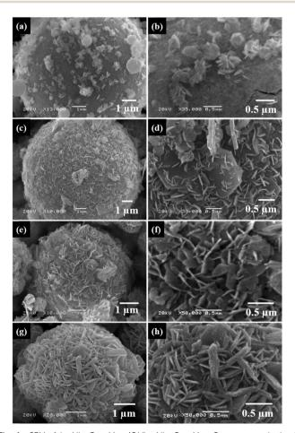
Fig. 4 SEM of the  $Ni_{0.8}Co_{0.1}Mn_{0.1}(OH)_2@Ni_{0.8}Co_{0.1}Mn_{0.1}O_x$  precursor obtained at different time intervals during the co-precipitation reaction: (a and b) 0.5 h; (c and d) 1 h; (e and f) 1.5 h; (g and h) 2 h.
