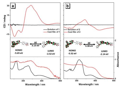
Fig. 1 UV and CD spectra of  $\bf{1}$  (a) and  $\bf{2}$  (b) in THF solution (10  $\mu$ M) and in the film state. Inset: HOMO and LUMO energy levels of  $\bf{1}$  (a) and  $\bf{2}$  (b).
