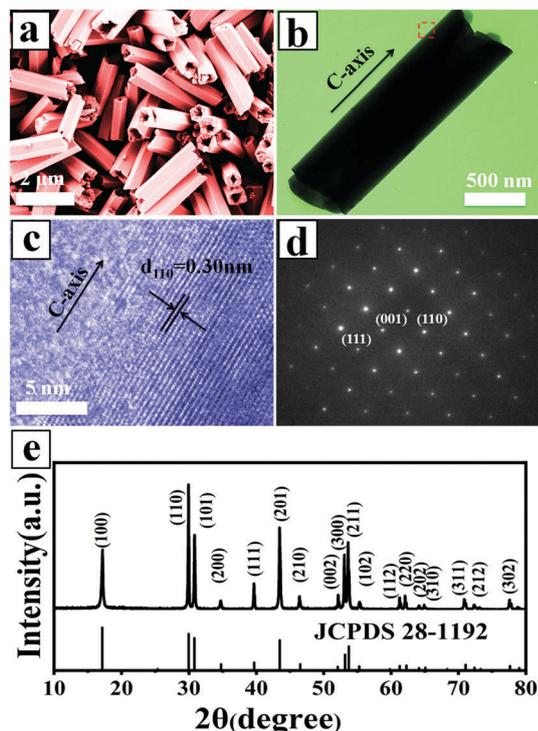
**Fig. 1** (a) FE-SEM image of the UCHMs-G sample, (b) TEM image of a single UCHMs-G microtube, (c) HR-TEM image taken from the area marked by the red rectangle in part b, (d) the corresponding SAED pattern of the UCHMs-G and (e) XRD pattern of the UCHMs-G with the standard data of  $\beta$ -NaYF<sub>4</sub> (JCPDS No. 28-1192) as a comparison.
