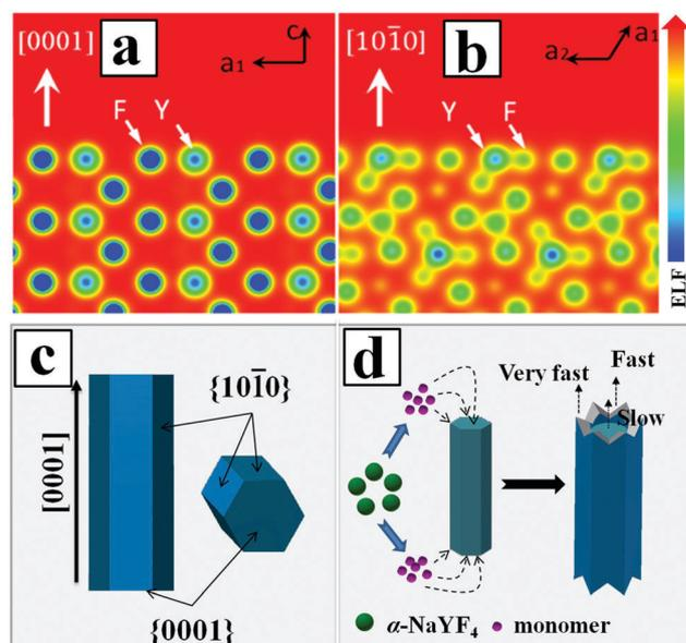
**Fig. 5** Maps of the electron localization function (ELF) for (a) the  $\{0001\}$  facet and (b) the  $\{10\bar{1}0\}$  facet, (c) schematic presentation of the  $\{0001\}$  and  $\{10\bar{1}0\}$  facets of hexagonal phase NaYF<sub>4</sub> and (d) illustration of the formation of microtubes with hollow structures and crown-like top ends.
