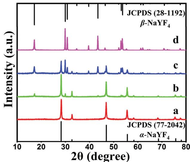
Fig. 3 XRD patterns of the intermediates obtained at different reaction time intervals: (a) 1 h, (b) 2 h, (c) 8 h and (d) 24 h, as well as the standard data of  $\alpha\text{-NaYF}_4$  (JCPDS No. 77-2042) and  $\beta\text{-NaYF}_4$  (JCPDS No. 28-1192) phases for comparison.
