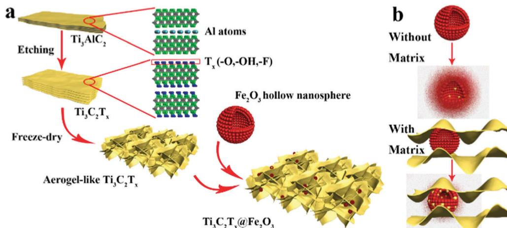
**Scheme 1** (a) Schematic illustration of the synthesis procedure for the Ti<sub>3</sub>C<sub>2</sub>T<sub>x</sub>@Fe<sub>2</sub>O<sub>3</sub> nanocomposite. (b) The mechanism of the MXene matrix protection in the Ti<sub>3</sub>C<sub>2</sub>T<sub>x</sub>@Fe<sub>2</sub>O<sub>3</sub> nanocomposite.
