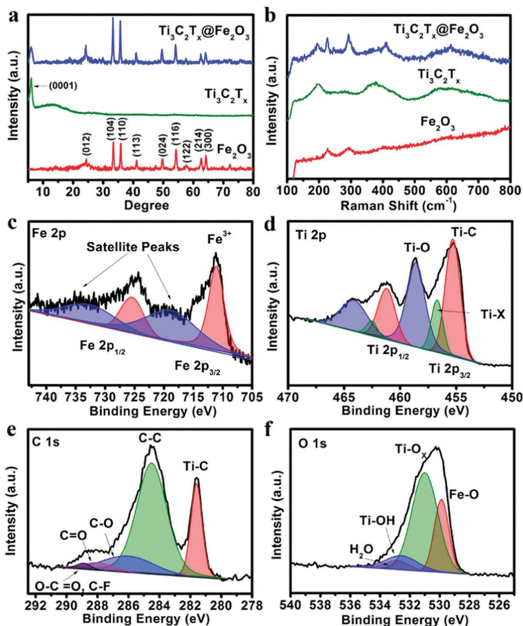
Fig. 1 (a) XRD patterns and (b) Raman spectra of the  $\text{Fe}_2\text{O}_3$ ,  $\text{Ti}_3\text{C}_2\text{T}_x$  and  $\text{Ti}_3\text{C}_2\text{T}_x@\text{Fe}_2\text{O}_3$  samples. (c) Fe 2p, (d) Ti 2p, (e) C 1s, and (f) O 1s XPS spectra of the  $\text{Ti}_3\text{C}_2\text{T}_x@\text{Fe}_2\text{O}_3$  nanocomposite.
