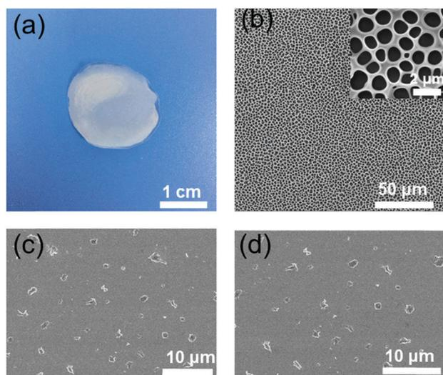
**Fig. 5** (a) Digital photo of the honeycomb-patterned films made from a solution of **A**<sub>2</sub>-**B**<sub>3</sub> complexes in CHCl<sub>3</sub> at the concentration of 7.5 wt% using the BF method; (b) SEM of the honeycomb-patterned films. (c and d) SEM images of films made from a solution of **A**<sub>2</sub>-**B**<sub>3</sub> complexes in CHCl<sub>3</sub> at the concentration of 7.5 wt% after adding 1.0 equiv. DTT using the BF method.
