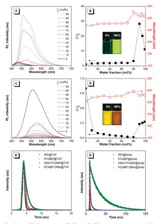
**Fig. 2** (A and C) PL spectra in THF and THF/water mixtures with different water fractions ( $f_{\rm w}$ ) of (A) DMA-POABP and (C) POABP-DMA. (B and D) Change in relative emission intensity ( $I/I_{\rm o}$ ) and emission maximum *versus* the water fraction of the THF/water mixtures of (C) DMA-POABP and (D) POABP-DMA.  $I_{\rm o}$  is the emission intensity in pure THF. (E and F) Fluorescence decay curves of POABP, DMA-POABP and POABP-DMA in (E) THF and (F) the solid state.
