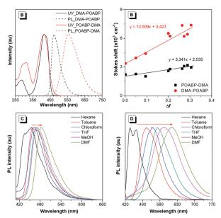
Fig. 1 (A) Normalized UV-vis absorption and PL spectra of the organoboron compounds in THF (10  $\mu\text{M})$ . (B) Lippert–Mataga plots of Stokes shifts versus the solvent orientation polarizability of DMA-POABP and POABP-DMA. (C and D) Normalized PL spectra of (C) DMA-POABP and (D) POABP-DMA in different solvents.
