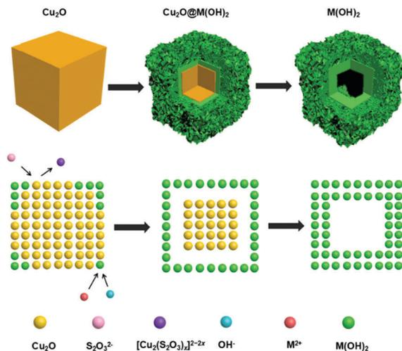
Fig. 1 Schematic illustration of the morphology evolution of  $M(\text{OH})_x$  ( $M = \text{Fe}, \text{Co}, \text{Ni}$ ) hollow nanocubes prepared through the Pearson's principle-inspired strategy and using  $\text{Cu}_2\text{O}$  nanocubes as the sacrificial templates.
