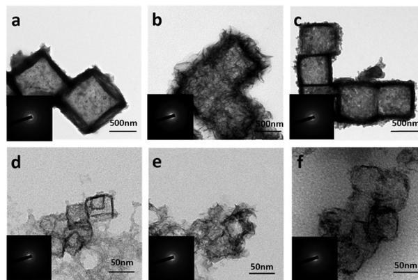
Fig. 2 TEM and SAED (inset) images of the as-prepared (a) Fe(OH)<sub>3</sub> (500 nm), (b) Co(OH)<sub>2</sub> (500 nm), (c) Ni(OH)<sub>2</sub> (500 nm), (d) Fe(OH)<sub>3</sub> (50 nm), (e) Co(OH)<sub>2</sub> (50 nm), and (f) Ni(OH)<sub>2</sub> (50 nm) hollow nanocubes.
