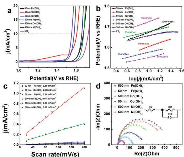
Fig. 4 Electrochemical properties of various hollow metal hydroxide nanocubes toward the OER in 1 M KOH solution. (a)  $J$ - $V$  curves after  $iR$  correction in comparison to an  $\text{IrO}_2$  commercial catalyst, (b) Tafel plots, (c) plots showing the extraction of the  $C_{dl}$  values, and (d) Nyquist plots (inset shows the equivalent circuit).
