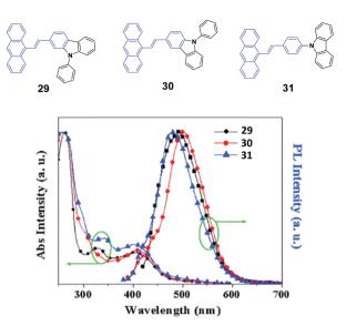
Fig. 10 (Top) The molecular structures of compounds 29, 30 and 31. (Bottom) The normalized absorption and PL emission spectra of vacuum deposited 29, 30, and 31 films. Reproduced with permission from ref. 49. Copyright 2016 Elsevier.
