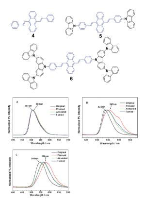
Fig. 4 (Top) The molecular structures of compounds 4, 5 and 6. (Bottom) The normalized PL spectra of 4 (A), 5 (B) and 6 (C) samples obtained under different conditions. Original: original sample; ground: ground sample; annealed: after annealing the ground sample at 200  $^{\circ}\text{C}$  for 5 min; and fumed: after fuming the ground sample in CH<sub>2</sub>Cl<sub>2</sub> vapor for 5 min. Reproduced with permission from ref. 32. Copyright 2012 American Chemical Society.
