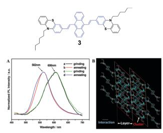
Fig. 3 (Top) The molecular structure of compound 3. (Bottom) (A) Normalized PL spectra of 3: (a) grinding, (b) annealing (a) at 100 °C for 1 min, (c) grinding, and (d) annealing (c) at 100 °C for 1 min. (B) Molecular packing of luminogen 3 in the single crystal structure. Adapted with permission from ref. 28. Copyright 2011 American Chemical Society.
