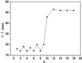
**Fig. 5** (Top) The molecular structure of compound **11**. (Bottom) Wavelength change of the luminogen **11** series *versus n* after grinding. Data from ref. 34.
