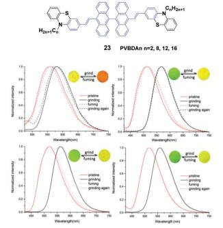
Fig. 8 (Top) The molecular structure of compound 23. (Bottom) Normalized fluorescence spectra of (a) PVBA2, (b) PVBA8, (c) PVBA12 and (d) PVBA16 in the solid state under external stimuli. Inset: Schematic diagrams of photos under 365 nm light. Reproduced with permission from ref. 46. Copyright 2015 The Royal Society of Chemistry.
