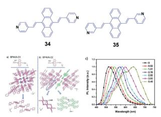
Fig. 11 (Top) The molecular structures of compounds 34 and 35. (Bottom) The aggregation state of 34 in the two single crystals: (a) C1 and (b) C2. (c) Normalized solid-state PL spectra of the 34 powder after the application of pressure (GPa). Reproduced with permission from ref. 52. Copyright 2013 The Royal Society of Chemistry.
