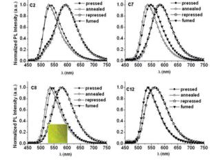
Fig. 7 (Top) The molecular structure of compound 20. (Bottom) Normalized emission spectra of IACn samples upon external stimuli (excited at 470 nm). Inset: A piece of filter paper soaked with IAC8 on which a rabbit is drawn using a metal spatula and illuminated under UV light. Reproduced with permission from ref. 43. Copyright 2015 The Royal Society of Chemistry.
