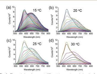
Fig. 4 The emission changes at different temperatures during the formation of the nanorods. (a) 15  $^{\circ}$ C, (b) 20  $^{\circ}$ C, (c) 25  $^{\circ}$ C, and (d) 30  $^{\circ}$ C.  $C_{\text{CTAB}} = 1.0 \text{ mg mL}^{-1}$ . The spectra were recorded every 3 min.
