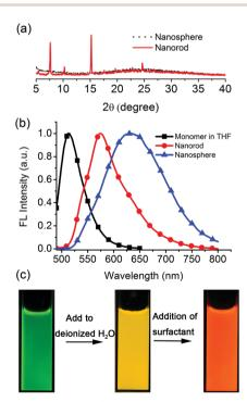
Fig. 2 (a) The XRD patterns of the nanospheres and nanorods. (b) The emission spectra of the BF<sub>2</sub>bcz monomer in THF, aqueous dispersions of the nanospheres and the nanorods. (c) The fluorescence images of the BF<sub>2</sub>bcz monomer in THF (left), aqueous dispersions of nanospheres (middle) and nanorods (right) under illumination with a UV lamp.
