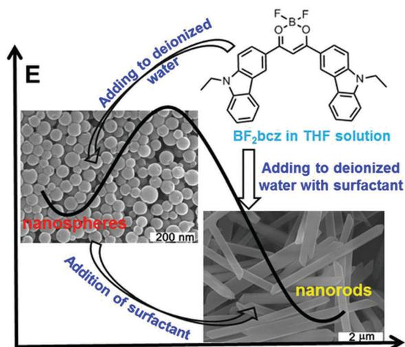
**Fig. 1** The image representation of the preparation of the  $\text{BF}_2\text{bcz}$  nanospheres and nanorods from the  $\text{BF}_2\text{bcz}$  monomer in THF solution, the morphological transition from nanospheres to nanorods, and the schematic energy diagram depicting the energy barrier between the nanospheres and nanorods.
