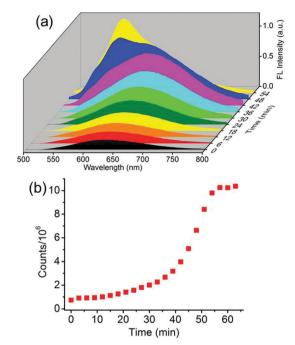
Fig. 3 (a) The emission changes during the morphological transition from nanospheres to nanorods by adding CTAB (1.5 mg mL<sup>-1</sup>) to the agueous dispersion of nanospheres. (b) The time-dependent emission intensities monitored at  $\lambda = 580$  nm during the process of nanosphere-nanorod transition.
