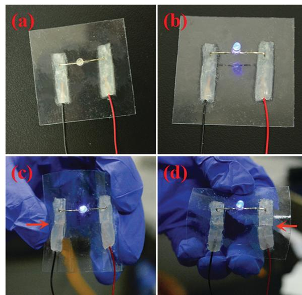
Fig. 5 Self-healing circuit based on hydrogel **HG**: (a and b) optical images of circuit based on **HG** hydrogel film at open and closed states; (c and d) the circuit functions well under bended and fractured states.
