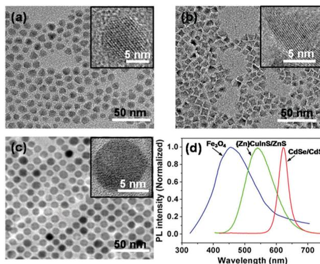
**Fig. 1** Typical TEM images of CdSe/CdS QDs (a), (Zn)CuInS/ZnS QDs (b) and Fe<sub>3</sub>O<sub>4</sub> nanoparticles (c). The insets in (a)–(c) are the HRTEM images of the QDs. (d) PL spectra of the QDs in THF.
