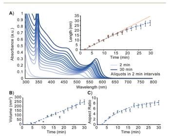
Fig. 1 Evaluation of unseeded CdSe nanorod growth. (A) UV-Vis at 2 min intervals over the first 30 min of nanorod growth. Nanorod dimensions measured using TEM analysis as a function of time are plotted for length (A, inset), volume (B), and aspect ratio (C). The equation for the line of best fit for the volume vs. time relationship is y = 9.7919x - 44.591. Associated TEM images are included in Fig. S1 (ESI†).
