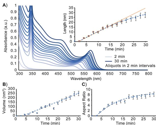
**Fig. 1** Evaluation of unseeded CdSe nanorod growth. (A) UV-Vis at 2 min intervals over the first 30 min of nanorod growth. Nanorod dimensions measured using TEM analysis as a function of time are plotted for length (A, inset), volume (B), and aspect ratio (C). The equation for the line of best fit for the volume vs. time relationship is  $y = 9.7919x - 44.591$ . Associated TEM images are included in Fig. S1 (ESI†).
