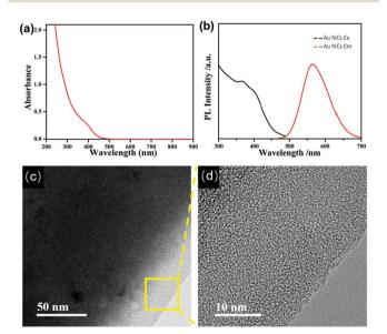
Fig. 1 UV-vis absorption spectrum (a), photoexcitation ( $\lambda_{em}$  = 565 nm, black line) and photoemission ( $\lambda_{\rm ex}$  = 365 nm, red line) spectra of the Au NCs (b). (c) TEM image of the Au NCs at pH 2.0. (d) HRTEM image of the zone marked by the yellow frame in (c).
