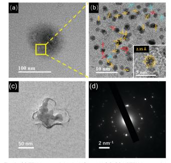
Fig. 4 (a) TEM image of the Au NCs at pH 8.0. (b) HRTEM image of the zone marked by the yellow frame in (a). (inset) Enlarged HRTEM image of one Au NC in (b). (c) Cryo-TEM image of the GNC solution at pH 8.0 and (d) the selected-area electron diffraction (SAED) of the aggregate.
