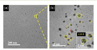
Fig. 5 (a) TEM image of the Au NCs at pH 11.0. (b) HRTEM image of the zone marked by the yellow frame in (a). (inset) Enlarged HRTEM image of the Au NCs in (b).
