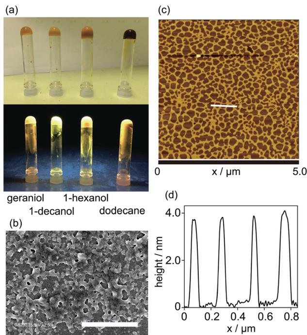
**Fig. 3** (a) Photographs of organogels of **1** (top) under daylight and (bottom) under UV light. (b) The FE-SEM image of the xerogel of **1**. Scale bar displays are 20  $\mu\text{m}$ . (c) The AFM image of **1**. (d) The height profile of the white line in (c).
