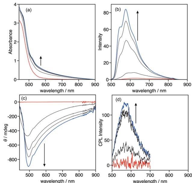
Fig. 5 Temperature-dependent (a) UV-vis absorption, (b) emission, (c) CD, and (d) CPL spectra of **1** in 1-decanol. The spectra were recorded every 10 °C. The arrows indicate the change in the spectra as the temperature decreases from 50 to 10 °C. Red and blue lines display the spectra at 50 and 10 °C, respectively.  $[\mathbf{1}] = 9.2 \times 10^{-3} \text{ mol L}^{-1}$ ,  $\lambda_{\text{ex}} = 430 \text{ nm}$ ;  $l = 0.1 \text{ cm}$ .
