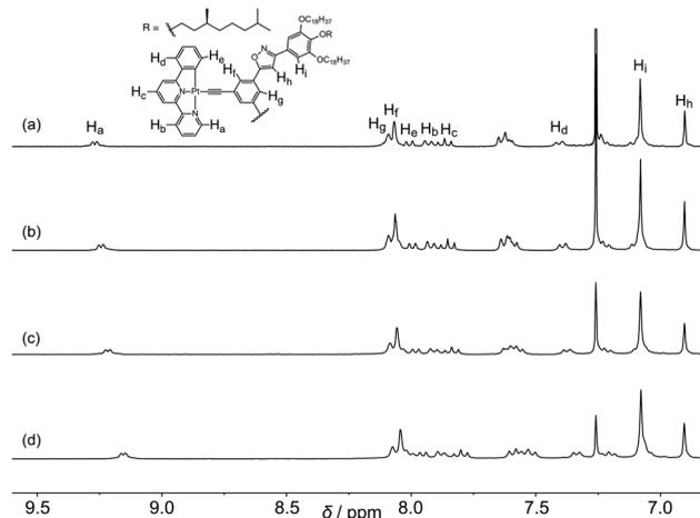
**Fig. 2** Concentration-dependent <sup>1</sup>H NMR spectra of **1** at 25 °C in chloroform-*d*. The concentrations of **1** are (a) 3.0, (b) 4.7, (c) 7.1, and (d) 14.2 mmol L<sup>-1</sup>.
