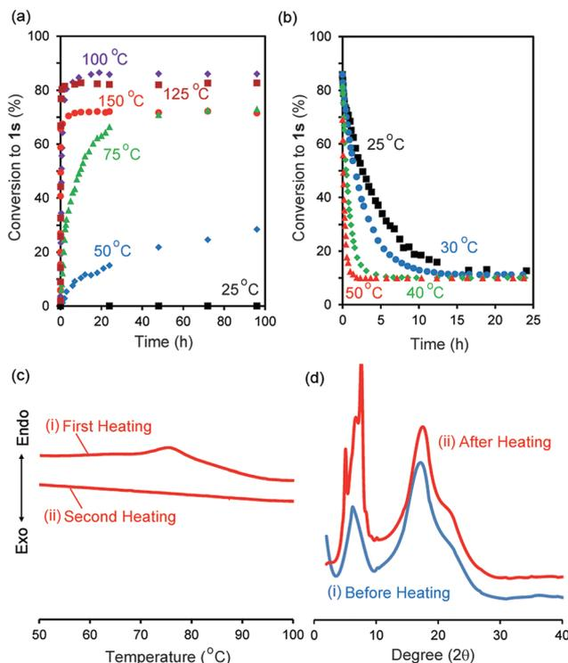
**Fig. 3** Percentage conversions to **1s** versus time (a) in solid state **1d** at 25 °C (black squares), 50 °C (blue diamonds), 75 °C (green triangles), 100 °C (purple diamonds), 125 °C (brown squares), 150 °C (red circles) and (b) in CDCl<sub>3</sub> at 25 °C (black squares), 30 °C (blue circles), 40 °C (green diamonds), 50 °C (red triangles). (c) DSC heating curves in (i) first and (ii) second heating processes. (d) PXRD patterns (i) before and (ii) after heating at 100 °C for 48 h.
