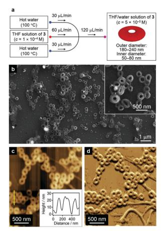
Fig. 8 (a) Schematic illustration of a microflow device used for the preparation of nanorings of 3, which are formed at higher temperatures. (b) The SEM image of the nanorings of 3 prepared by using this microflow device. (c and d) AFM height (c) and phase (d) images of the thus prepared nanorings of 3 [the inset in (c) shows the cross-sectional analysis along the yellow line].
