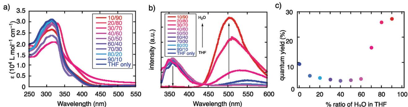
Fig. 2 Photophysical properties of **TBFE** in a THF/H<sub>2</sub>O mixed solvent system. (a) Absorption spectra ( $1.0 \times 10^{-5}$  M), (b) fluorescence spectra ( $1.0 \times 10^{-6}$  M,  $\lambda_{\text{ex}} = 317$  nm), and (c) transition of photoluminescence quantum yield measured by the absolute method.
