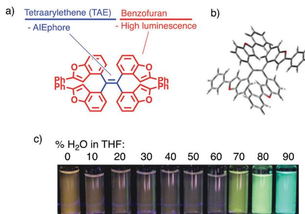
Fig. 1 Tetrakis(benzo[*b*]furyl)ethene (**TBFE**). (a) Molecular design. (b) Crystal structure showing twisting around the TAE centre (see ESI†). (c) Fluorescence intensity dependent on THF/H<sub>2</sub>O ratio (excitation at 365 nm).
