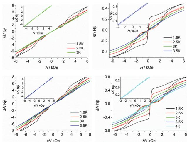
**Fig. 12** Field dependence of the normalized magnetization of samples **2** (top left), **2b** (top right), **de1** (bottom left) and **de1b** (bottom right) between 1.8 and 4 K at a sweep rate of 200 Oe s<sup>-1</sup>. Inset: *M* versus *H* plots for each at the highest temperature.
