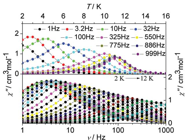
Fig. 4 Temperature (up) and frequency  $\nu$  (down, logarithmic scale) dependence of out-of-phase ( $\chi''$ ) ac susceptibility in the temperature range 2–16 K for **1** under a zero dc field.
