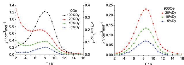
**Fig. 7** Temperature dependence of the out-of-phase susceptibility ( $\chi''$ ) at 100 Hz and applied fields of (left) 0, and (right) the optimum field 900 Oe for the diluted samples **1a**, **1b** and **1c**.
