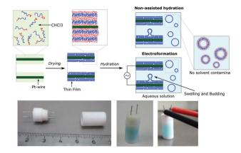
Fig. 2 Electrochambers and electroformation methodology. Scheme of non-assisted film hydration and electroformation methods. (b) Picture of the open homemade electro-chamber (left), the closed chamber after filling here with aqueous sucrose solution doped with AF<sup>647</sup> as used in the non-assisted film hydration method (middle) and then connected to the generator for electroformation (right).
