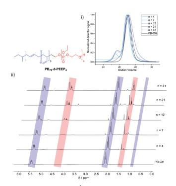
Fig. 1 Stacked GPC curves: (i)  $^{1}$ H NMR spectra and (ii) of PB-OH and PB<sub>73</sub>-b-PEEP<sub>n</sub> with the corresponding signal assignments.
