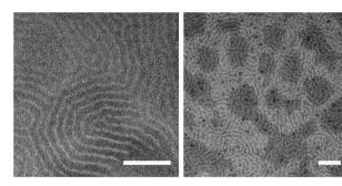
Fig. 6 Transmission electron microscopy (TEM) of  $PB_{73}$ -b- $PEEP_{21}$  films stained with  $RuO_4$  exhibiting extensive lamellar networks. Scale bar: 100 nm.
