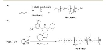
Scheme 1 Synthesis of polybutadiene-b-poly(ethylene ethyl phosphate) (PB-b-PEEP). (a) Initial living anionic polymerization of butadiene to generate hydroxyl terminated 1,4-rich polybutadiene (PB(1,4)-OH). (b) Organocatalyzed anionic ring-opening polymerization of ethylene ethyl phosphate to the amphiphilic block copolymers PB-b-PEEP.
