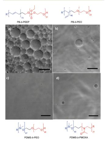
Fig. 3 Typical phase contrast microscopy image of (a)  $PB_{73}$ -b- $PEEP_{12}$ , (b)  $PB_{46}$ -b- $PEO_{23}$ , (c)  $PDMS_{67}$ -b- $PEO_{48}$ , and (d)  $PDMS_{60}$ -b- $PMOXA_{21}$  by film hydration. Scale bar: 100  $\mu$ m.
