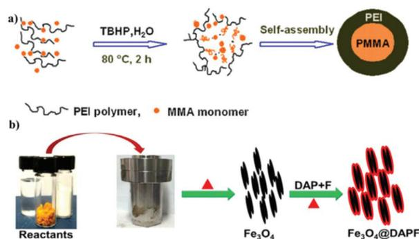
**Fig. 1** (a) Synthesis of PMMA/PEI core-shell nanoparticles. Reproduced with permission from ref. 37. Copyright 2011 Elsevier. (b) Schematic illustration of the Synthesis of Fe<sub>3</sub>O<sub>4</sub>@DAPF ferromagnetic nanorods. Reproduced with permission from ref. 38. Copyright 2015 American Chemical Society.
