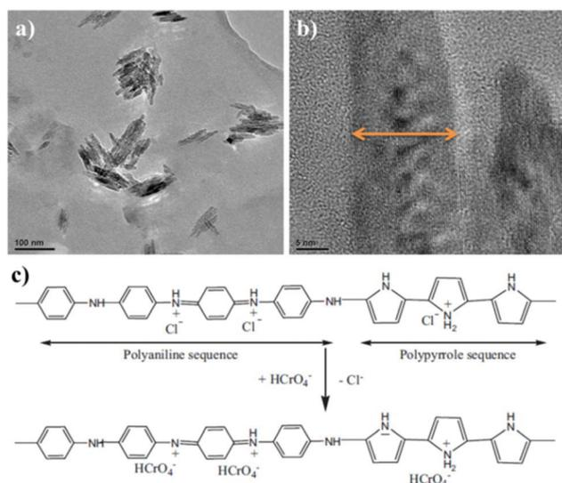
**Fig. 4** (a) and (b) High-resolution TEM images of the PPy-PANI nanofibers at two different magnifications. (c) Plausible pathway to remove Cr(VI) from aqueous solutions using the PPy-PANI nanofibers. Reproduced with permission from ref. 68. Copyright 2012 Elsevier.
