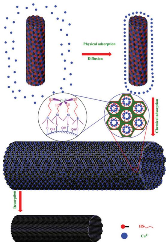
Fig. 6 The mechanism of Cu(II) adsorption on PVA/SiO<sub>2</sub> nanofibers. Reproduced with permission from ref. 92. Copyright 2010 Elsevier.
