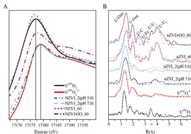
**Fig. 9** XANES spectra (A) and Fourier transform (FT) of EXAFS spectra (B, solid and dashed lines: experimental and fitted data) for reference samples and U(VI)-reacted nZVI and nZVI/rGO composites, *T* = 25 ± 1 °C, *I* = 0.01 mol L<sup>-1</sup> NaClO<sub>4</sub> pH = 5.0. Reproduced with permission from ref. 174. Copyright 2014 Elsevier.
