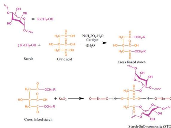
Fig. 2 Synthesis of starch/SnO<sub>2</sub> nanocomposites. Reproduced with permission from ref. 55. Copyright 2016 Elsevier.
