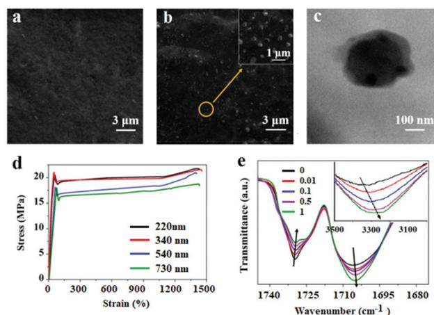
**Fig. 2** SEM images of (a) blank DAPU and (b) DAPU-PDAP composites (PDAP content: 1 wt%); (c) typical TEM image of PDAPs in DAPU-PDAP composites (PDAP content: 1 wt%); (d) effect of PDAP particle size on the tensile properties of DAPU-PDAP-1 with 1 wt% PDAP content; (e) FTIR spectra of DAPU-PDAP composites with different contents of PDAPs (PDAPs size:  $\sim$ 340 nm).
