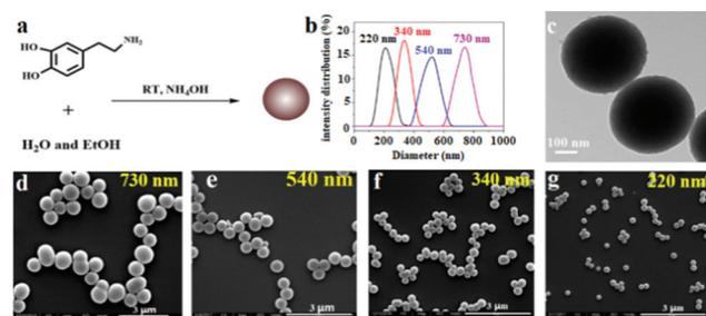
**Fig. 1** (a) Schematic illustration of the synthesis of PDAPs. (b) PDAP diameter distribution statistical analyzed from SEM images by Nano Measurer 1.2. (c) Typical TEM image of PDAPs with an average diameter of 340 nm. (d-g) SEM images of PDAPs with different diameters prepared at different ratios of ammonia to dopamine.
