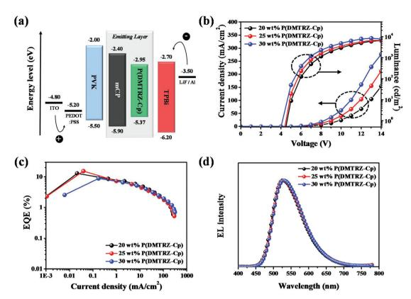
Fig. 4 (a) Schematic energy level diagram of a device with mCP as the host, (b) current density-voltage-luminance (J-V-L) curves, (c) external quantum efficiency (EQE)-current density ( $\eta_{\text{ext}}$ -J) curves and (d) electroluminescence (EL) spectra at a luminance of 1000 cd m<sup>-2</sup> of TADF-OLEDs fabricated using the new P(DMTRZ-Cp) polymer emitter.
