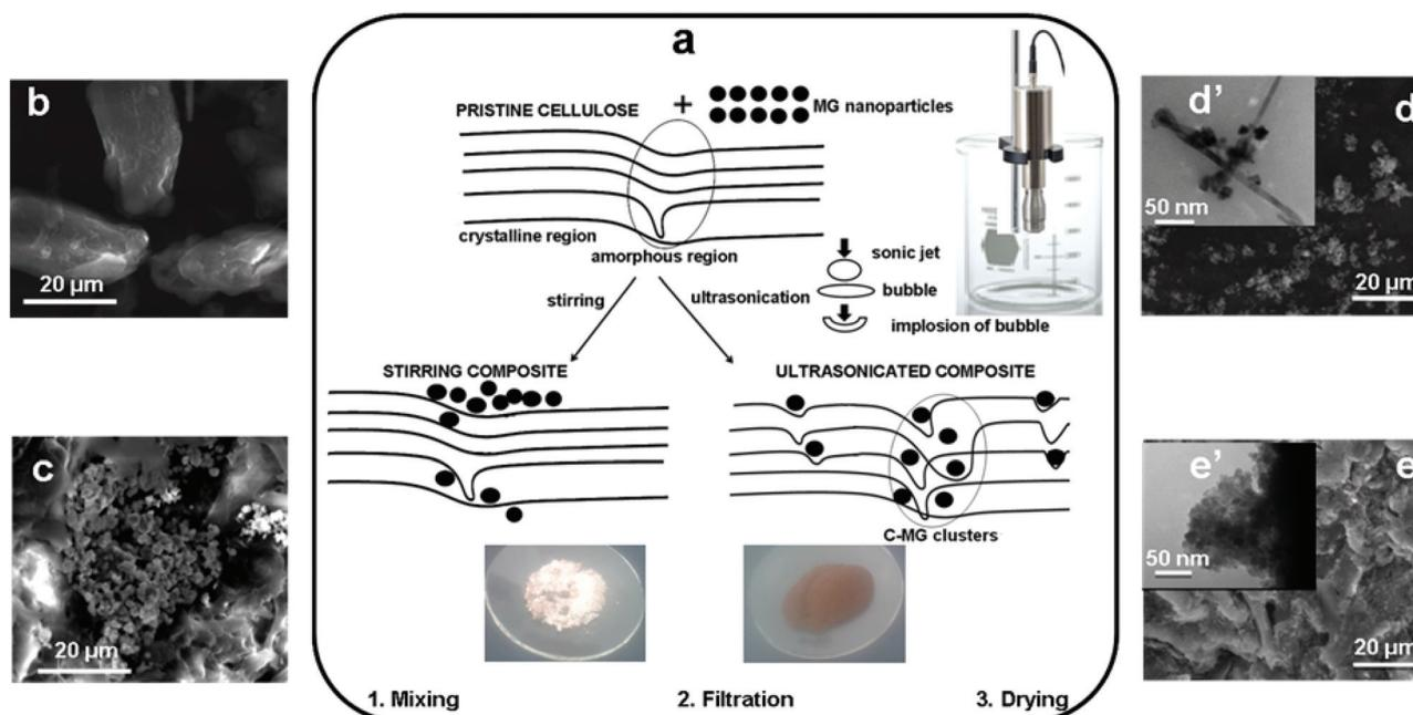
**Fig. 1** Overview of the preparation of cellulose–maghemite/goethite composites: (a) schematic representation of the preparation methods and of the microstructures of C-MG composites obtained by stirring and ultrasonication; the effect of the combined action of ultrasonication and nanoparticles on the crystalline structure of cellulose is highlighted: SEM images of (b) pristine cellulose, (c) C-MGst (d), MG and (e) C-MGultr; TEM images of (d') MG and (e') C-MGultr.
