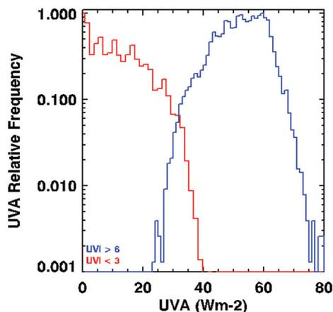
Fig. 2 Frequency distribution of UVA ( $y$ -axis, normalised to unity in each case) for the case where UVI is less than 3 (red), and for the case where UVI is greater than 10 (blue). The data used are the same as shown in Fig. 1 (*i.e.*, daytime scans only). In nearly 5–10% of cases, the UVA for UVI < 3 is greater than that for UVI > 10.
