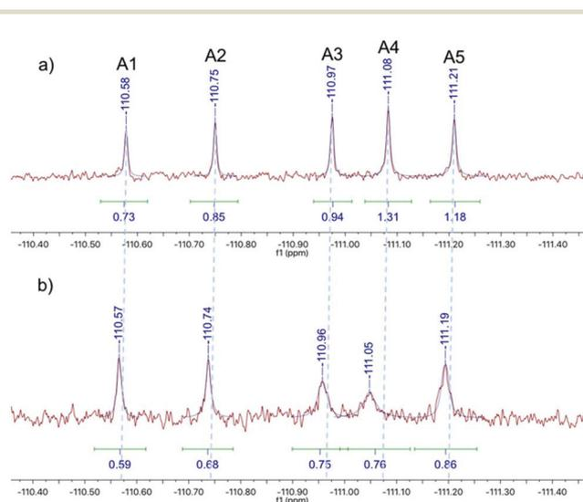
Fig. 4  $^{19}\text{F}$  NMR spectra of the  $^{19}\text{F}$ -labelled DCL: (a) the DCL equilibrated in the absence of the protein target, (b) the protein-templated DCL equilibrated in the presence of FabH.
