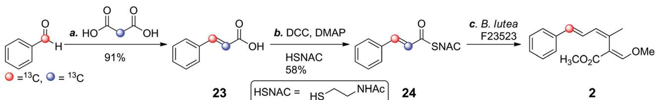
**Scheme 2** Reagents and conditions: (a)  $[2-^{13}\text{C}]$ -malonic acid (1.02 equiv.),  $\text{Na}_2\text{SO}_4$  (0.15 equiv.), pyridine, piperidine, reflux, 4 h, 91%; (b) DCC (1.13 equiv.), DMAP (0.04 equiv.), HSNAC (1.43 equiv.), DCM, 0 °C, 2 h, 23 °C, 16 h, 58%.
