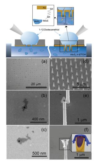
Fig. 1 SEM micrographs of  $MoS_2$  flakes deposited onto an array of plasmonic nanoholes. (Top panel) Illustration of the concept for controlled deposition of  $MoS_2$  flakes over metallic holes; (a) top view over a large flat gold hole array; (b) and (c) details of a single-layer flake on a 2D pore; (d) tilted view over a large array of 3D antennas covered with  $MoS_2$  flakes; (e) and (f) details of the  $MoS_2$  flakes deposited onto an antenna.
