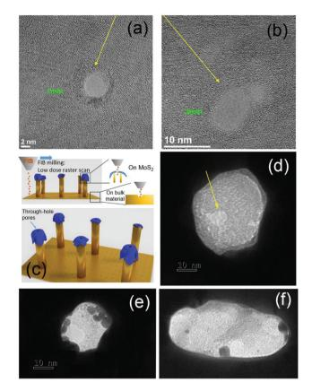
Fig. 4 (a) TEM micrograph of a nanohole sculptured into a MoS<sub>2</sub> layer by means of HRTEM exposure for 1 minute; (b) TEM micrograph of a nanohole sculptured into the MoS<sub>2</sub> layer by means of HRTEM exposure for 3 minutes; (c) illustration of the concept used for FIB milling of the MoS<sub>2</sub> nanopore array; (d) example of a nanopore prepared by means of FIB; (e) and (f) examples of AuNPs grown on a MoS2 layer(s) after FIB milling.
