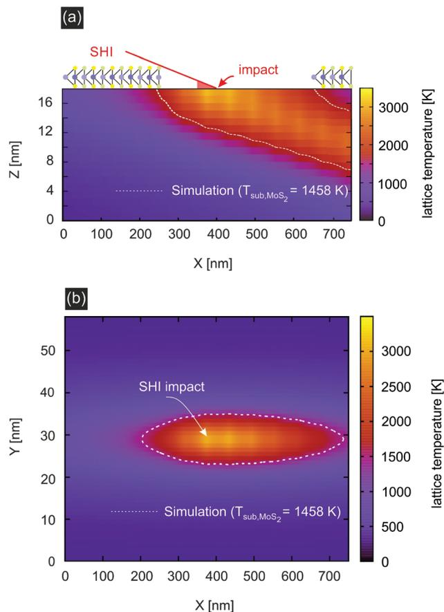
Fig. 4 Calculated temperature profile (a) side and (b) top view in the SiO<sub>2</sub> substrate after irradiation with 91 MeV Xe ions under a grazing incidence of 1° with respect to the surface. The white dotted line depicts the isotherm at the decomposition temperature of MoS<sub>2</sub>.
