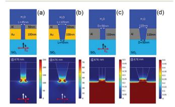
Fig. 2 Sketch of a section of the ideal and fabricated rectangular Au-Al (top panels a-b) and of the circular Al (top panel c-d) nanoslot. Nearfield intensity distributions of the Au-Al (bottom panels a-b), and Al nanoslots (bottom panels c-d) (ideal and fabricated) at the experimental wavelength. The maximum of the colorbar does not correspond to the field maximum. The section planes of the rectangular slots are parallel to the short axis.
