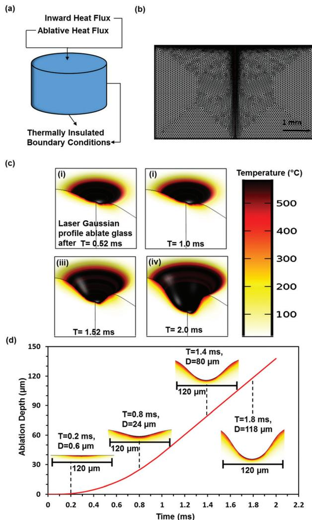
**Fig. 1** The simulated  $\text{CO}_2$  laser ablation process of the soda lime glass. (a) The geometry created to simulate the glass substrate with the applied boundary conditions. (b) The meshed geometry. (c) Temperature and 3D cavity profile variations with time; (i) 0.52 ms, (ii) 1.0 ms, (iii) 1.52 ms, and (iv) 2.0 ms. (d) The ablation depth of the concavity as a function of the laser processing time.
