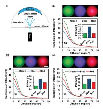
Fig. 4 Light scattering from optical diffusers. (a) Schematic setup for recording a 3D diffusion pattern. (b-d) Diffusion plots of the doublesided surface relief devices analyzed using different wavelengths ( $\lambda_1$  = 450 nm,  $\lambda_2$  = 533 nm, and  $\lambda_3$  = 633 nm), with their respective diffraction patterns captured using a circular semi-transparent white globe. (a) Grid (HD = 20  $\mu$ m), (b) grid (HD = 30  $\mu$ m), and (c) parallelogram patterns. Scale bar = 6 cm.
