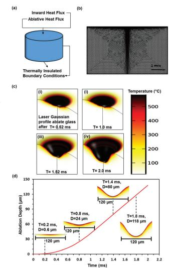
Fig. 1 The simulated CO<sub>2</sub> laser ablation process of the soda lime glass. (a) The geometry created to simulate the glass substrate with the applied boundary conditions. (b) The meshed geometry. (c) Temperature and 3D cavity profile variations with time; (i) 0.52 ms, (ii) 1.0 ms, (iii) 1.52 ms, and (iv) 2.0 ms. (d) The ablation depth of the concavity as a function of the laser processing time.
