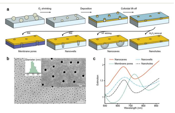
Fig. 1 Nanostructure fabrication and characterization. (a) Preparation of different plasmonic nanopores using colloidal lithography on various supports followed by different etching steps. (b) Electron microscopy imaging of nanopores from above with diameter distribution. (c) Extinction spectra of the different nanopores in water showing plasmon resonance peaks.
