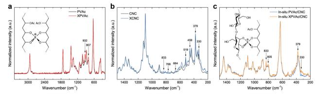
Fig. 3 (a) Raman spectra of PVAc and XPVAc films in a spectral range of 200-3500 cm<sup>-1</sup>, and the chemical structure of borax-crosslinked PVAc chains. (b) Raman spectra of CNCs and XCNCs in a spectral range of 200-1500 cm<sup>-1</sup>. (c) Raman spectra of in situ PVAc/CNC and in situ XPVAc/CNC films (weight ratio of PVAc to CNCs is 80:20), and a possible chemical structure of borax-crosslinked PVAc-CNCs.
