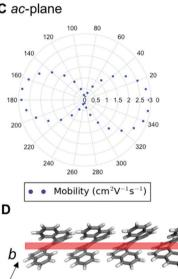
Fig. 8 Angular-dependent electron-mobility for structure 11 in the (a) ab-, (b) bc- and (c) ac-planes; (d) the adjacent translational homochiral chain (substructure type I) with electron-mobility of  $2.9~\text{cm}^2~\text{V}^{-1}~\text{s}^{-1}$ . The red arrow shows the highest electron-mobility direction for structure 11.
