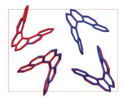
Fig. 4 An overlay of the experimental HEXHEL enantiopure structure (1) viewed down the c axis (red) and the lowest-energy computed [6]helicene crystal structure (blue), as relaxed with the B86bPBE-XDM method.
