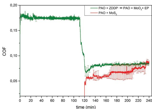
Fig. 5 Coefficient of friction as a function of time for the lubricant mixtures containing 5 wt% MoO<sub>3</sub> in combination with the 2 wt% EP additive when running on a ZDDP tribofilm pre-formed during the initial 2 hours of rubbing. The friction value obtained with a lubricant containing 5 wt% MoS<sub>2</sub> nanotubes is shown as a reference value.
