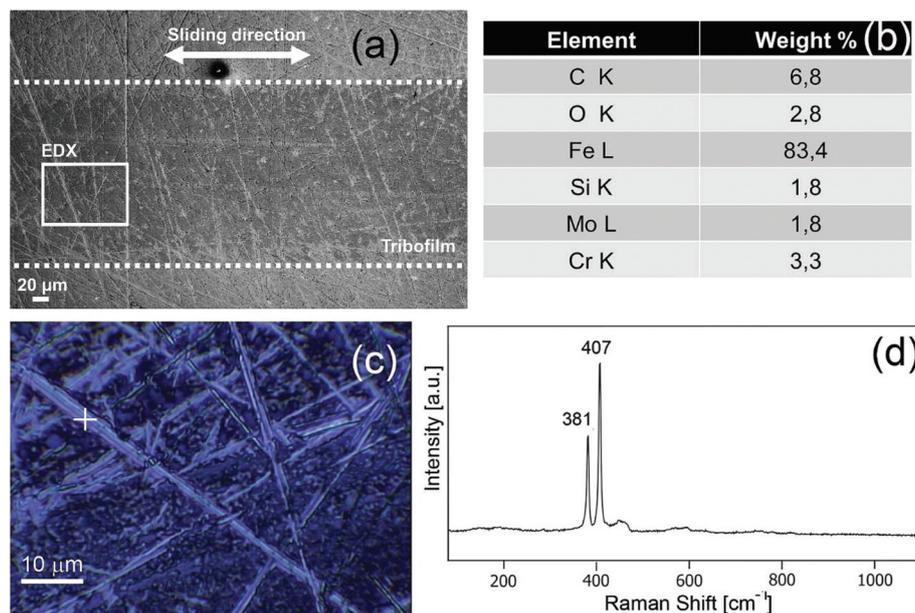
Fig. 4 Analyses of the sample lubricated with the mixture containing 5 wt% MoS<sub>2</sub> nanotubes: (a) wear scar showing a dark tribofilm using 2 kV acceleration voltage; (b) elemental composition of the tribofilm obtained by EDX; (c) position of the wear track (cross) where the Raman spectroscopy measurements were performed; (d) Raman spectrum with the characteristic peaks for MoS<sub>2</sub> at 381 and 407 cm<sup>-1</sup>.
