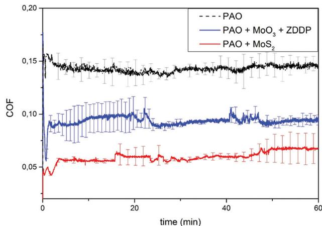
**Fig. 2** Coefficient of friction as a function of time for the lubricant mixtures containing 5 wt% MoO<sub>3</sub> nanotubes with the 2 wt% ZDDP anti-wear additive and 5 wt% MoS<sub>2</sub> nanotubes. The friction value obtained for pure PAO base oil is shown as a reference value.
